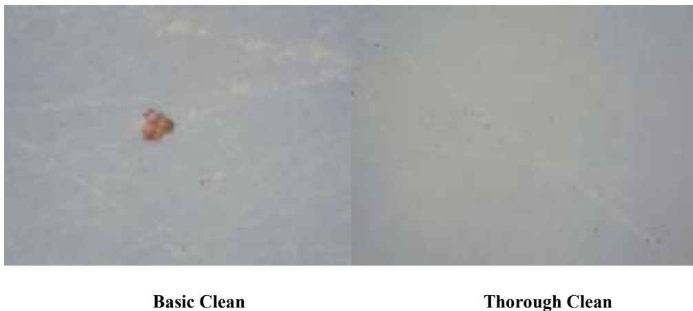
Figure R9. Photos illustrating effect of thorough clean on sample surface of PTFE
