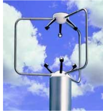
Figure 5. Sonic Anemometer These transducers send and receive sonic signals.
